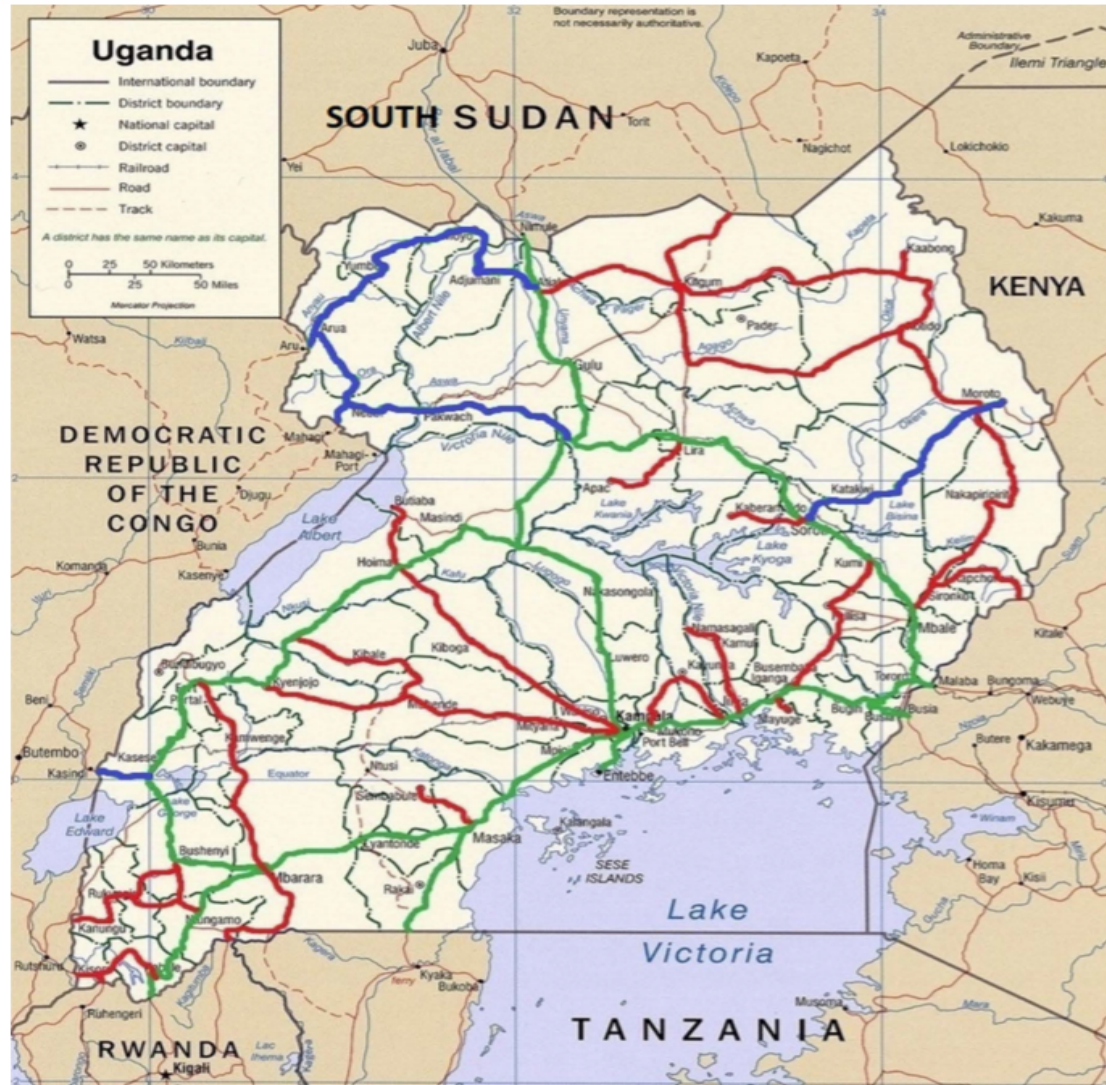
Fig 10: Map showing fibre-optic coverage of the NBI
