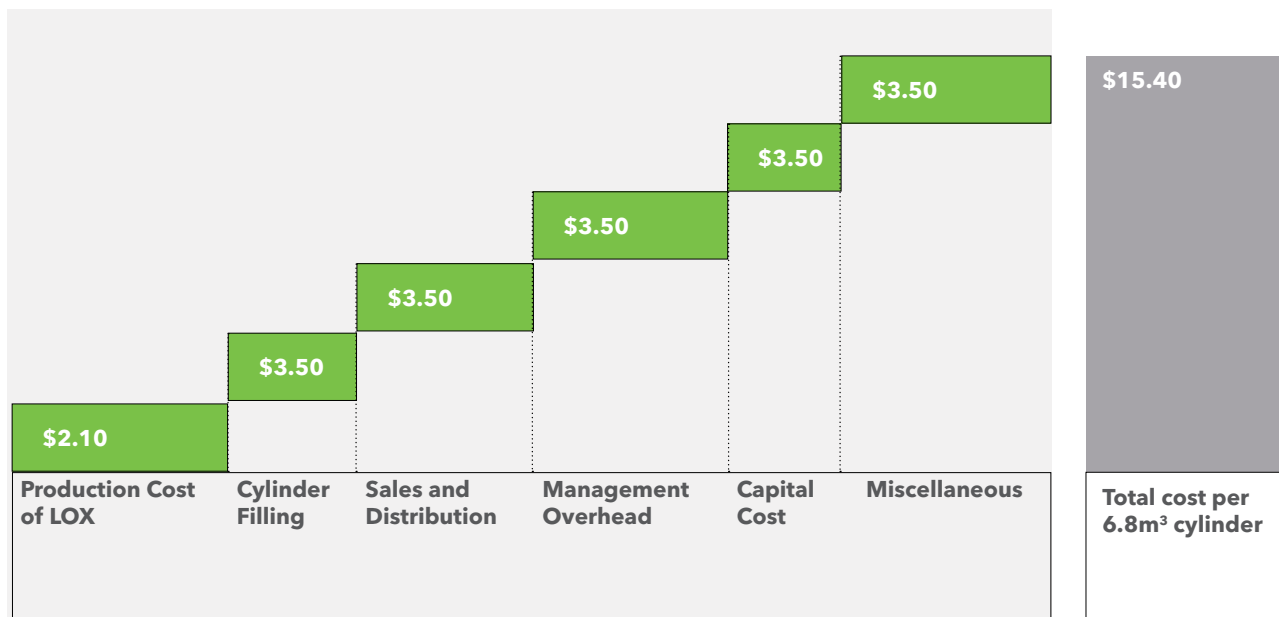
Figure 2: Cost of each 6.8 m3 oxygen cylinder at the point of use in clinics or hospitals
